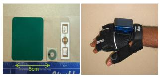
Figure 2: RFID Tags (L) and Glove-Based Reader (R)
