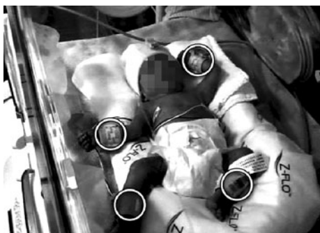
Fig. 1 Baby being monitored by 4 Eco accelerometers in the NICU (identified by the white circles )
